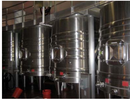
Wine tanks heated by captured cogen. heat
